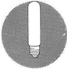
BURNING POSITION. The shaded portion of this diagram shows the position in which this lamp MUST NOT BE MOUNTED.
